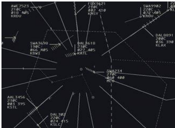
Fig.1. Example of how aircraft are displayed on a radar screen. Only a portion of the display is shown to better illustrate the aircraft and their associated data blocks. The full display can be found in Fig. 2 within the results and discussion section.
