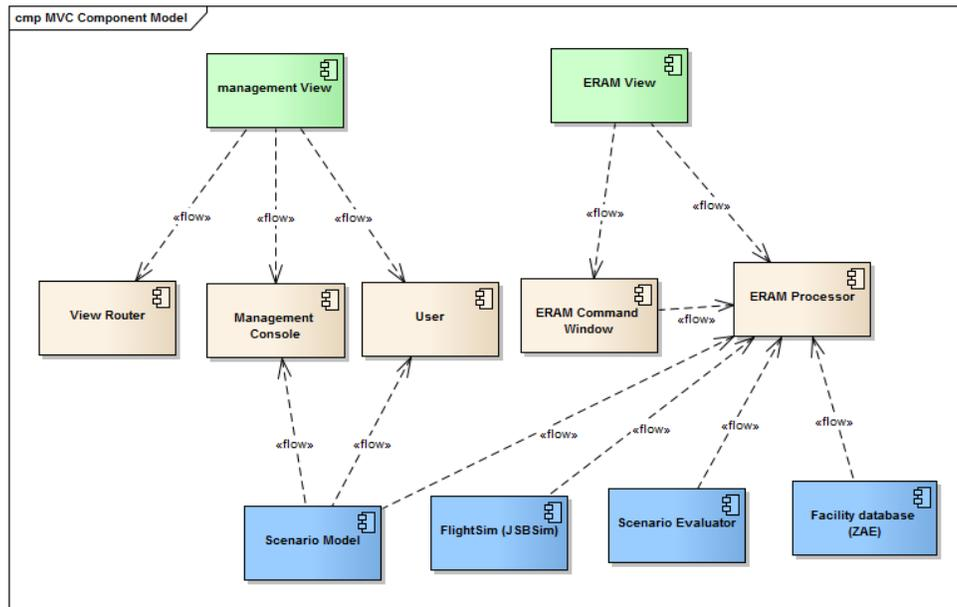
**Fig. 3 ASTT Model-View-Controller (MVC) High Level Architecture**
